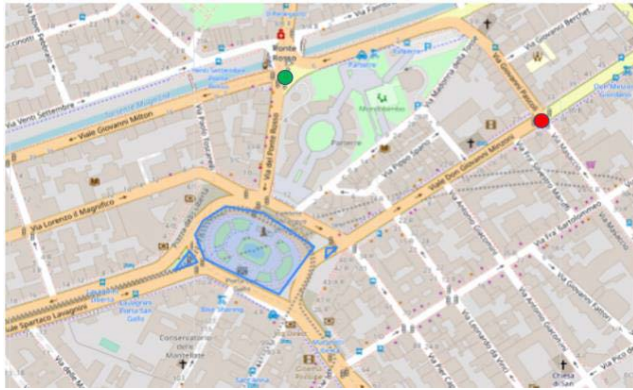
FIGURE 4. Scenario represents the real blocking area caused by the roadworks begun in December 2019 around “Piazza della Libertà” square due to future rail location in Florence. Red dot represents the location of the road graph network, having highest betweenness before the starting date of such works in the city, green dot stands for the position when graph road changes have been applied.
