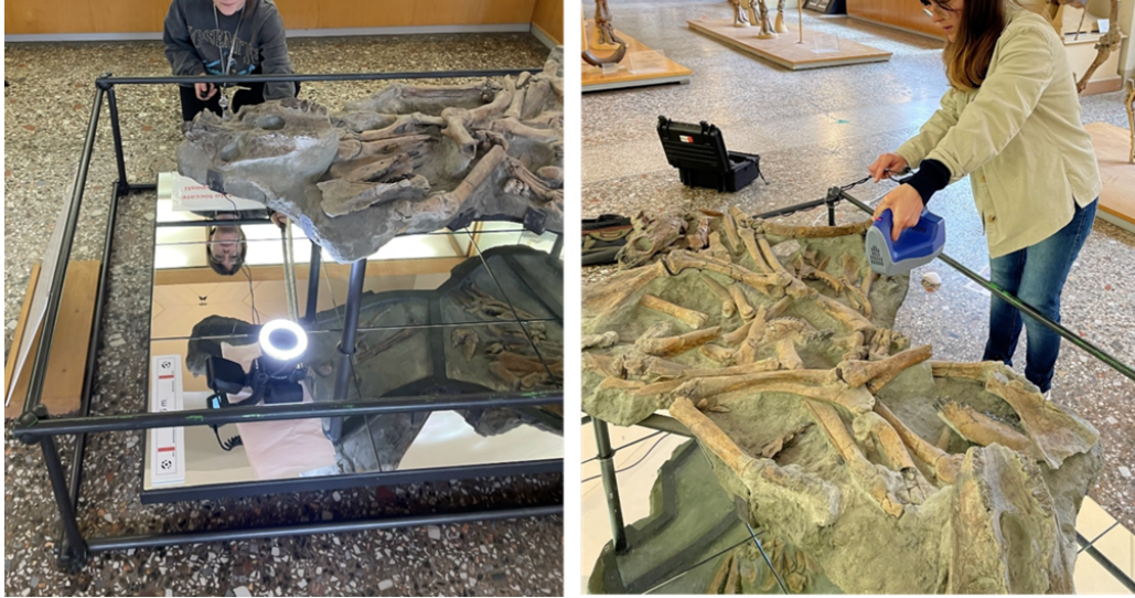
Figure 2.4: Digitisation attempts through photogrammetry (left) and light-structured scanning (right) of the whole fossiliferous block.
