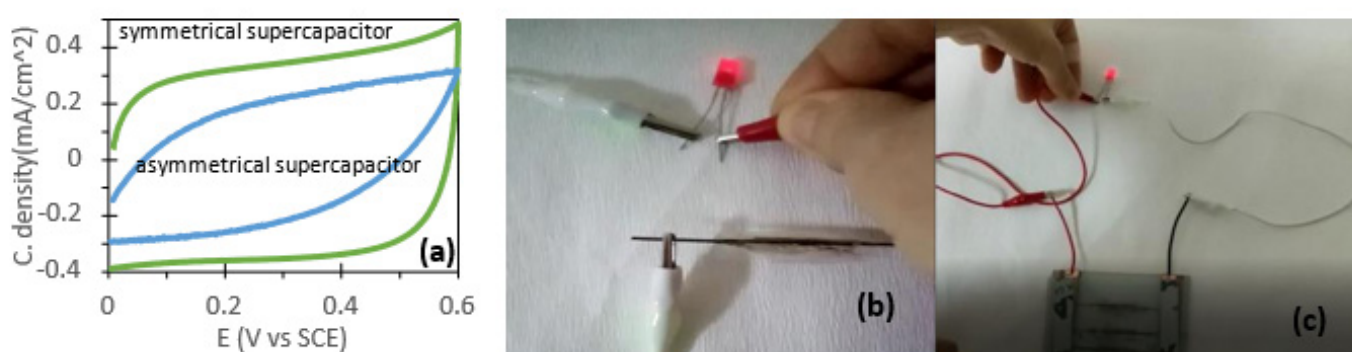
Figure 1. (a) CV curves of the symmetrical and asymmetrical supercapacitors, (b) symmetrical and (c) asymmetrical supercapacitors enlighten an LED.
