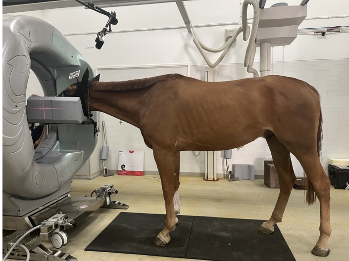
Figure 4.7: Illustrative standing equine CBCT workflow in which a lightweight ChArUco board is rigidly attached near the region of interest and observed by an auxiliary RGB camera for external pose tracking.
