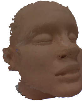
Figure 4.14: RGB–D pointcloud obtained with the Intel RealSense D435.
