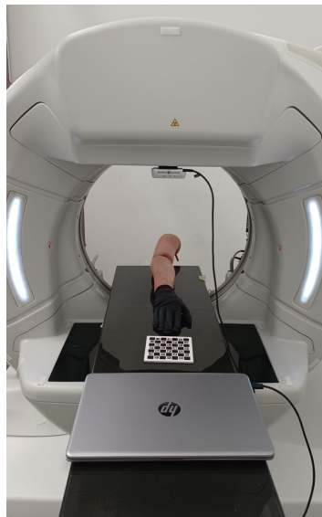
Figure 4.10: Optical scouting setup: Intel RealSense D435 mounted on the See Factor CT3 gantry; a ChArUco board provides a fiducial reference for multi-view alignment.
