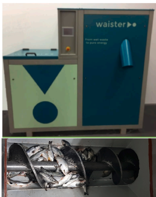
Fig. 4. “Waister 15 drying technology for mortalities” (Baarset et al., 2021).
