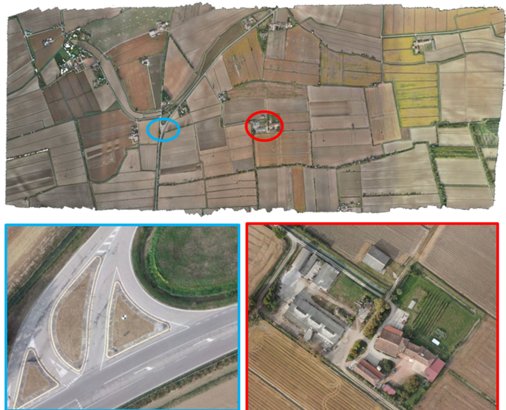
Figure 8. Ortophoto of the whole area obtained with Agisoft Metashape: simulation of a fast investigation of the overall situation of portions of the affected area surveyed during EXE 1.
