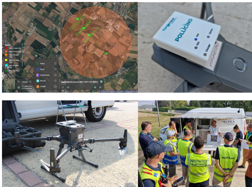
Figure 6. Some risk mitigations applied during UAS joint activity: NFZ visualized in D-flight with the drone trajectories in green (top left—images courtesy of Topview), drone tracker (top right and bottom left) and on-site meeting with all the UAS teams (bottom right).
