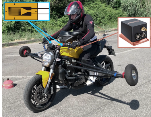
Figure 3. The instrumented motorcycle with outriggers, as used in the experiment. The positions of the inertial platform and strain gauges are shown.
