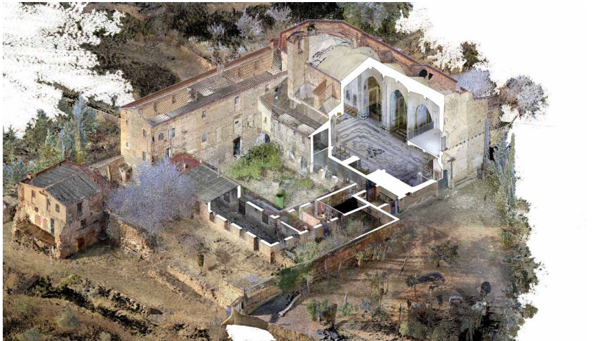
Fig. 5 Digital laser- scanner survey campaign of the hermitical caves.
