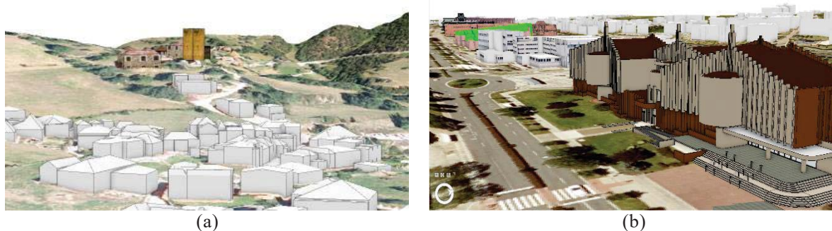
Fig. 2: Some examples of models generated. (a) GIS 3D of Mogrovejo (LoD 2-LoD 3). (b) GIS & HBIM integrated model (LoD 4-HBIM LOD 300) of Civil Eng. School - Univ. Cantabria.
