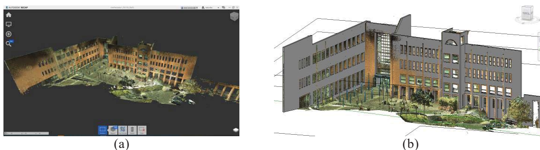
Fig. 2: (a) Point cloud in Autodesk Recap; (b) View of the HBIM model with the integrated point cloud.
