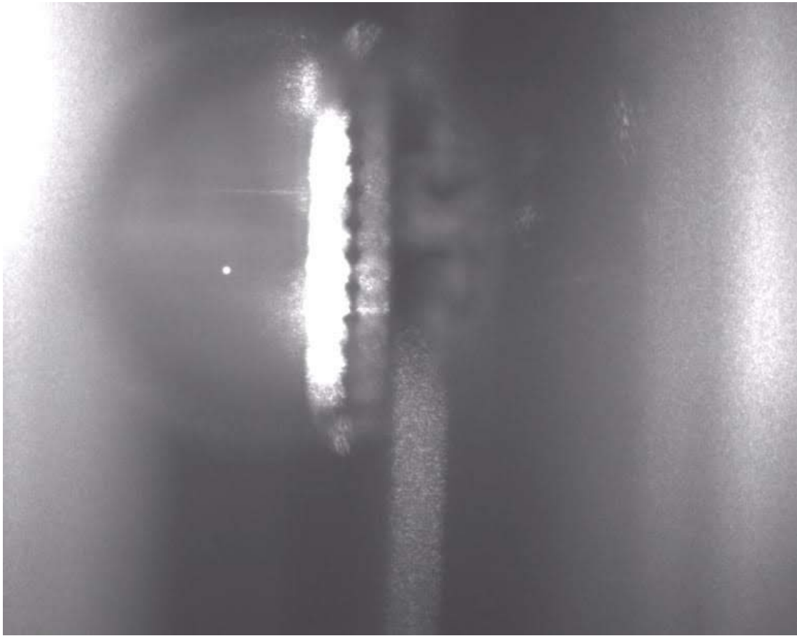
Figure 42: Top view of a nanoparticle levitating on the cavity axis in high vacuum.
