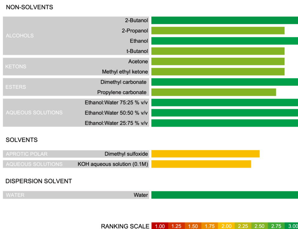
Figure 1. Graphical representation of the global score that averages, for each starch solvent and nonsolvent considered in the present study, the “green” scores provided by industrial and academic institutions. Nonsolvents also include blends of water and ethanol. The global scores were translated in colors ranging from deep red (lower end) to yellow (average values) and up to deep green (high end), as shown by the ranking scale on the bottom.
