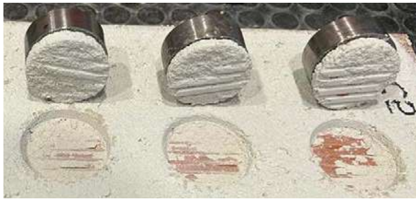
Fig. 5 Appearance of plaster C5 after tearing: the observed failure is of the cohesive type of the plaster in tests A) and B), in C) there was also partial fracture of the substrate.
