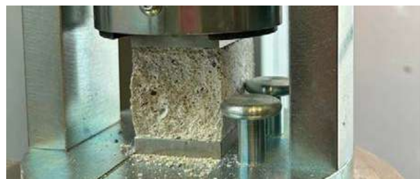
Fig. 4 Appearance of S3.5 after the compressive rupture
