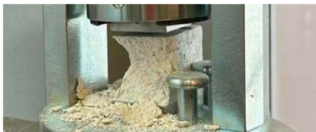
Fig. 3 Appearance of C3.5 after the compressive rupture.
