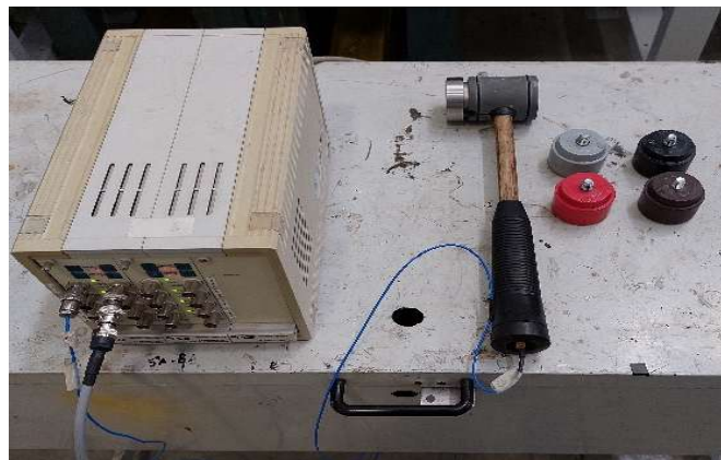
Figure 4.4: Instrumented hammer and amplifier used for the hammer test.
