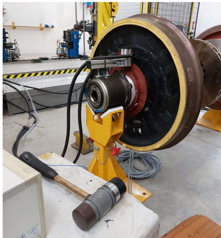
Figure 4.4: Instrumented hammer and amplifier used for the hammer test.
