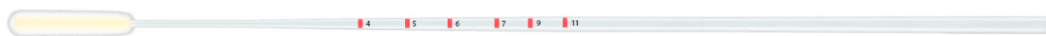
Figure 4. The newly designed nasopharyngeal swab, featuring marks along the shaft to signpost the proper depth of penetration along the nasal floor at different ages. The mark next to the number corresponding to the patient’s age should be aligned with the nostril.
