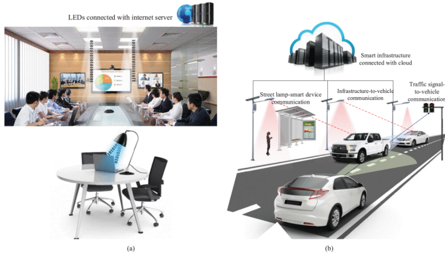
Figure 1.3: VLC application: a) Indoor VLC network, b) outdoor VLC based intelligent transport system (ITS). Reproduced from [1]
