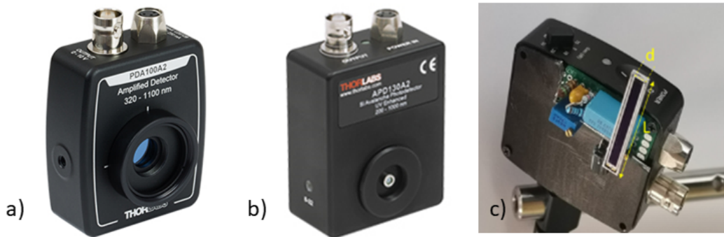
Figure 2.5: Image of Photodetectors. a) Photograph of Thorlabs PDA100A2. b) Photograph of Thorlabs APD 430 A/M ( c) Photograph of the Hamamatsu S3588-09 connected to the PDA100A2 TIA, used to collect the light from a thin FC slab.
