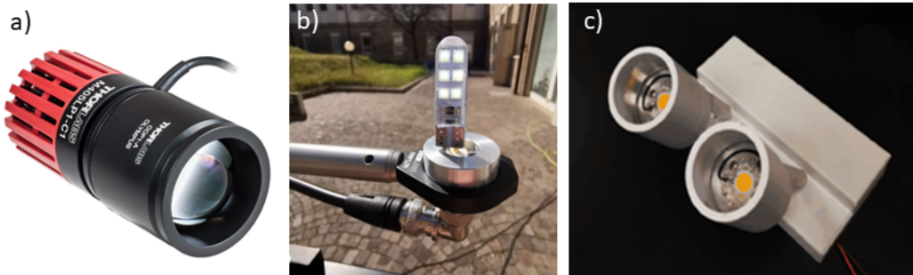
Figure 2.4: Images of main light sources used in experiments: a) 405 nm collimated light sources; b) automotive WLED; c) museum spotlight.
