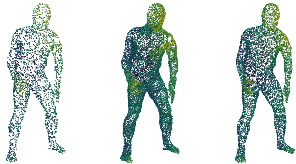
Figure 2: Left: Sample of an input low-resolution point cloud with \sim 3\text{K} vertices. Center: our model reconstruction with \sim 12\text{K} vertices. Right: Ground truth point cloud with \sim 12\text{K} vertices.
