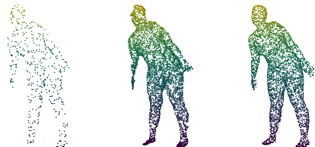
Figure 6: Left: Sample of a single frame from an input low resolution point cloud with ~512 vertices, Center: reconstruction obtained with our proposed solution; Right: Ground truth point cloud.
