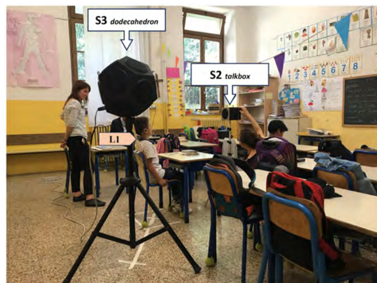
Figure 5. Experimental setup of binaural measurements in the classroom C1 (untreated): listener L1 and the two sources (S2, Talkbox at one meter from the listener L1 and dodecahedron S3, at one meter from the listener).
