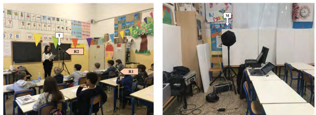
Figure 8. Experimental setup during the comprehension tests: on the (left), positions of the Talkbox (T) and microphones (R2 at one meter from the Talkbox, R1 in the middle) in the classroom C1; on the (right), positions of the masking sound source (dodecahedron) (M) in the classroom C2. In the photo the absorbing panels placed near the walls are shown.
