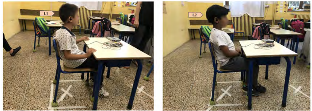
Figure 6. Experimental setup of binaural measurements in the classroom C1: on the (left), listener type one (L1); on the (right), listener type two (L2).
