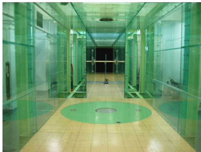
Figure 15: Wind tunnel in the Department of Civil and Earth Resources Engineering, Kyoto University, Japan (courtesy of Prof. Masaru Matsumoto and Prof. Hiromichi Shirato).
