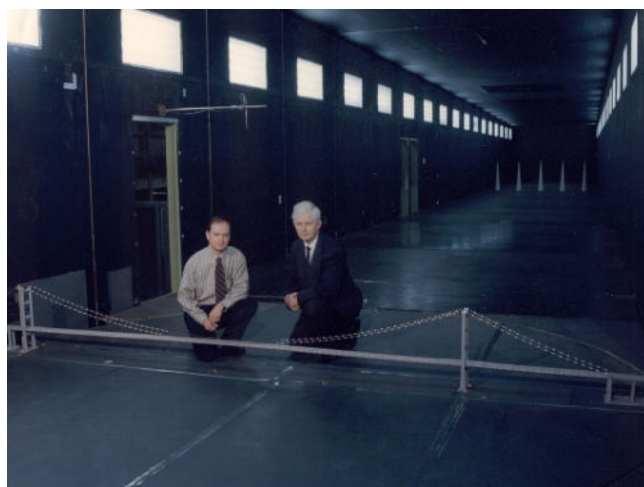
Figure 14: Alan G. Davenport (right) and J. Peter C. King (left) in the wind tunnel of the University of Western Ontario Laboratory, London, Canada, behind the 1:400 full-aeroelastic model of the Tsing Ma Bridge, Hong Kong, China (courtesy of the University of Western Ontario Laboratory).
