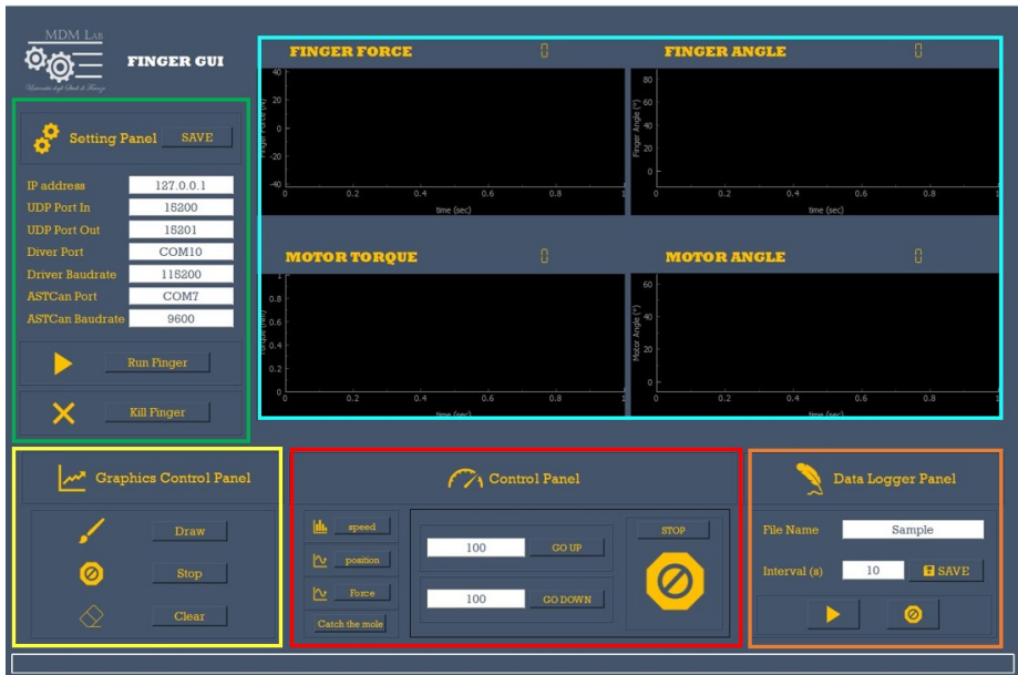
Figure 5.4: An overview of the Finger GUI with colored frames highlighting the various panels. Specifically: the setting panel, in green; the control panel, in red; the data logger panel, in orange; the graphics area, in blue; the graph control panel, in yellow; and the text box, in white.
