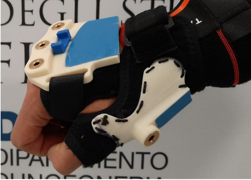
Figure 3.2: The BP module for the thumb is on the left, the BP for the long finger is on the right.
