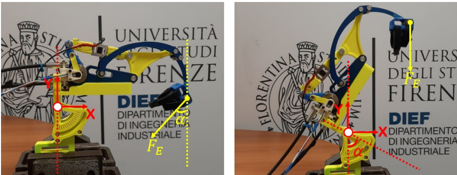
Figure 6.2: The custom bracket equipped with an adjustable orientation base.
