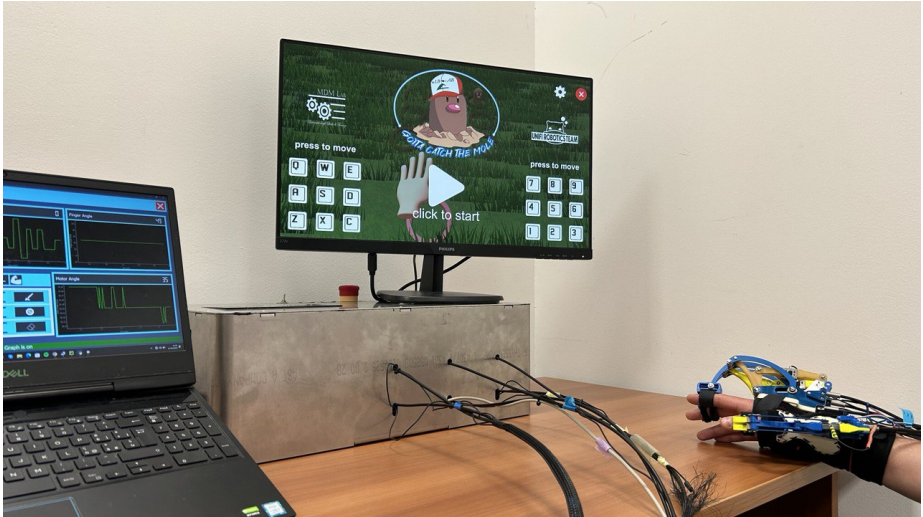
Figure 1.1: An overview of the HES presented during functioning via the custom-developed Finger GUI and Catch the mole application.
