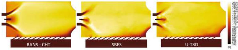
Figure 3.13: Temperature maps on XY midplane of the combustion chamber: RANS CHT (left), adiabatic SBES (Middle) and simplified U-THERM3D (right) simulations
