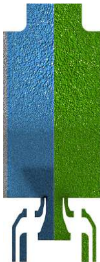
Figure 4.5: Visualization of the three mesh grids employed to discretize the involved calculation domains: gas-phase (blue), solid plates (gray) and radiation (green)
