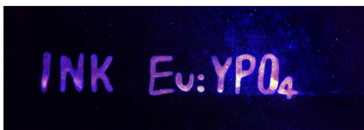
Figure 1. Ink 15% w/w Eu:YPO 4 in 10% w/w PVA 99+% hy under UV light (365 nm, 400W).
