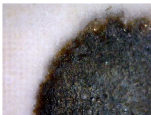
Figure 12 Black's fine grain in sample C18. Optical microscope in reflected light, 180x.
