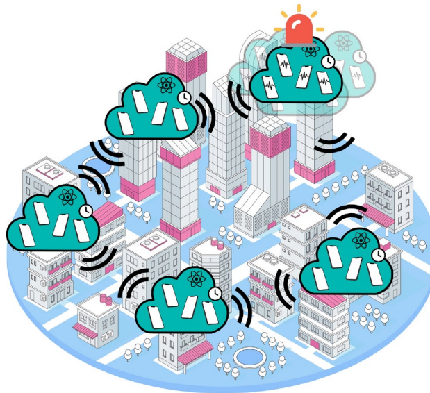
Figure 7. Sketch of the cluster of a synchronized network of mobile sensors. Each cluster is independent but it is interconnected to each other and a central station for calibration purposes (image freely modified from www.freepik.com contents).
