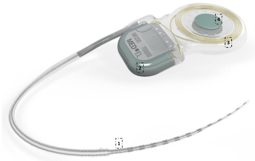
Figure 11. Internal components of the CI. The cochlear implant is made by the electrode array (1) that guarantee the patient to understand sound and speech. The array is connected to processor (2) that receive input from a communication link (3) and a multi-magnet assembly (4) that allow user to capture sounds and safely undergo high resolution imaging. (In this photo: a MED-EL cochlear implant)
