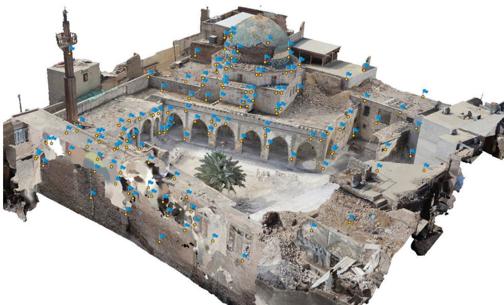
Figure 5: Three-dimensional view of the photogrammetric model used in surveys, displaying control points where the model was compared with the laser scanner point cloud.
