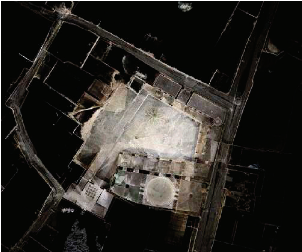
Figure 4: Orthoimage from the point cloud depicting the extent of the laser scanner survey of the religious complex.
