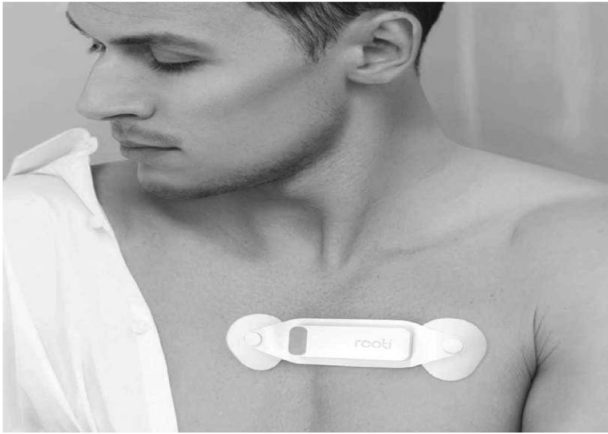
Fig. 1 The RootiRx. The RootiRx® multisensory patch-type system is a water-resistant compact ECG patch of 62 \times 22 \times 9 mm size and 14 g of weight. Published with permission from Rooti Labs Ltd.
