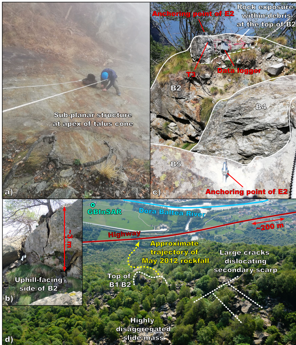
Fig. 5 a Sub-planar structure outcropping at the apex of the talus cone. b Evidences of brittle fracture damage on the uphill-facing side of block B2 c Close-up photograph of the upper S-facing lateral side of block B2 (taken from block B5, looking north), showing the anchoring points of tiltmeter T3 and extensometer E2 (downslope
