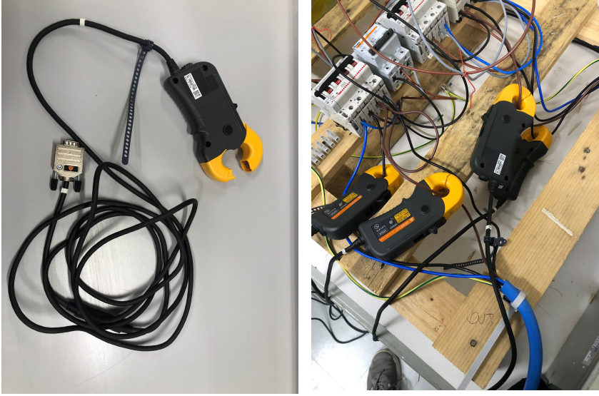
Figure 8.7: Dewesoft FLuxGate Transducers
