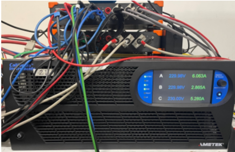
Figure 8.3: Ametek AC Programmable Source.
