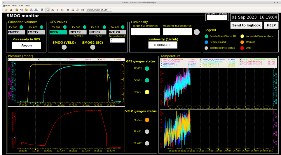
Figure III.3.14: SMOG2 monitoring panel at the end of a test injection in the VELO vessel; the pressure readings in the VELO vessel (red) and in the PZ601 (light blue) and PZ602 (yellow) can be seen in the bottom left frame, while the temperature in the storage cell and in the VELO vessel can be seen in the bottom right frame.
