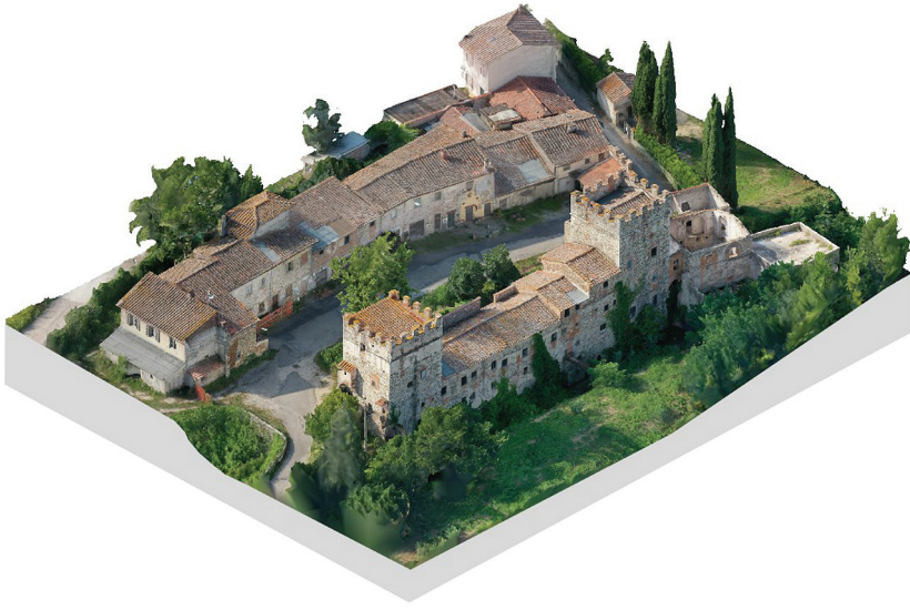
FIGURE 7 Three-Dimensional Model Obtained from the Photogrammetric Survey of the Complex
