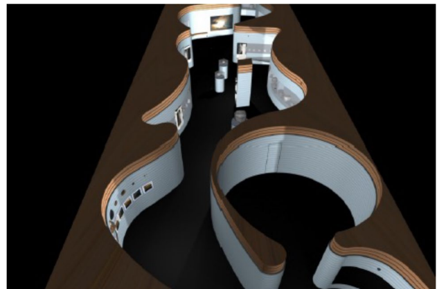
Fig. 3 A top-view 3D model of the curvilinear MISP's exhibition path. The image shows the ALUCOBOND® cladding sheets of the display walls and the fireproof wooden slats on the top of the primary vertical structure
