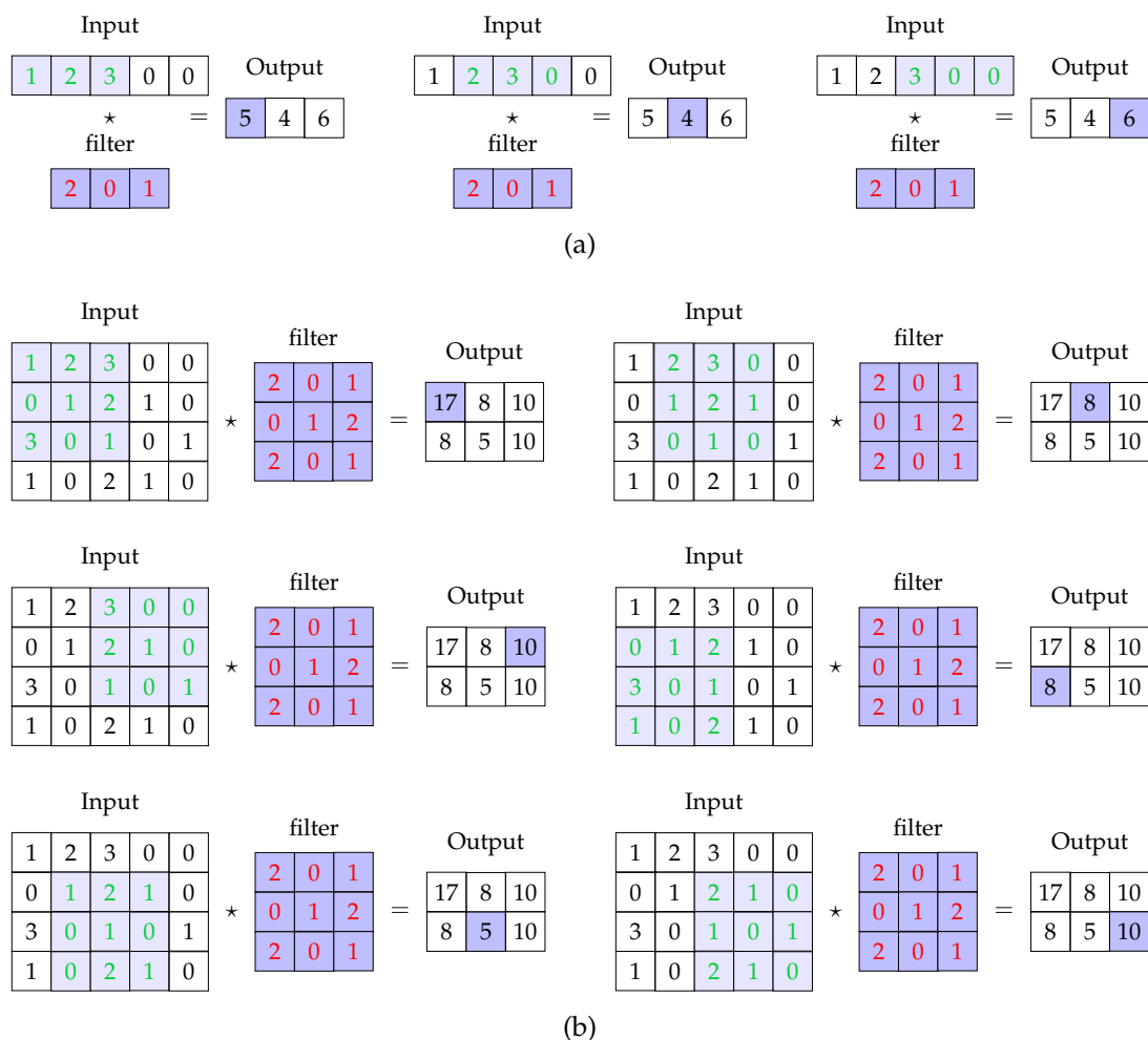
Figure 2.13: Examples of convolutional operators for 1D (a) and 2D (b).
