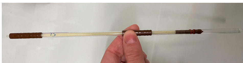
Figure 2.4: 5 mm shuttle tube employed with the fast shuttle system.
