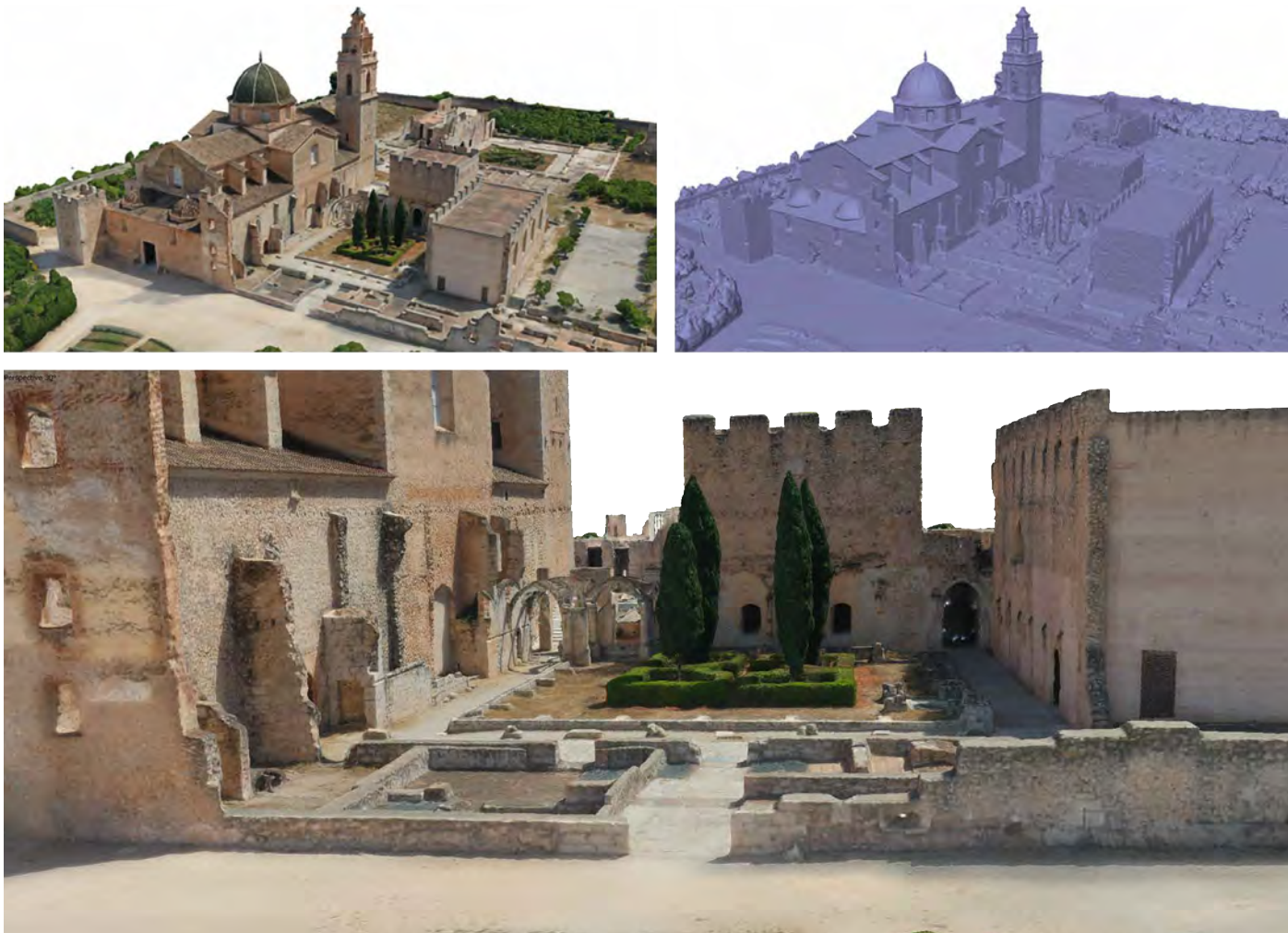
↑ Fig. 10 UAV Survey data Material and morphological quality of the photogrammetric data.
