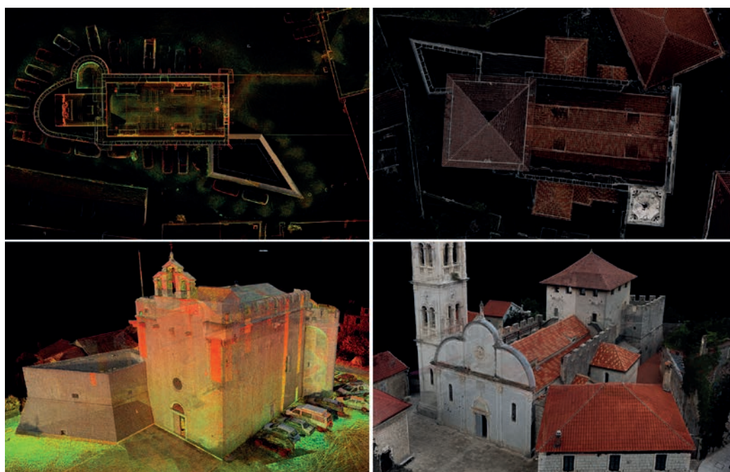
Fig. 3. Comparison between the fortified churches of St. Mary in Vrboska (left) and St. Mary in Jelsa (right). The point clouds provide an overall view of the ecclesiastical layout and its defensive apparatus, highlighting typological, morphological and construction-related similarities and differences within the fortified system of the island of Hvar.
