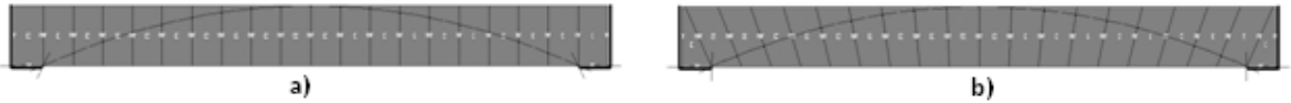
Figure 6. Flat arch: structural response as a function of the slope of the joints.
