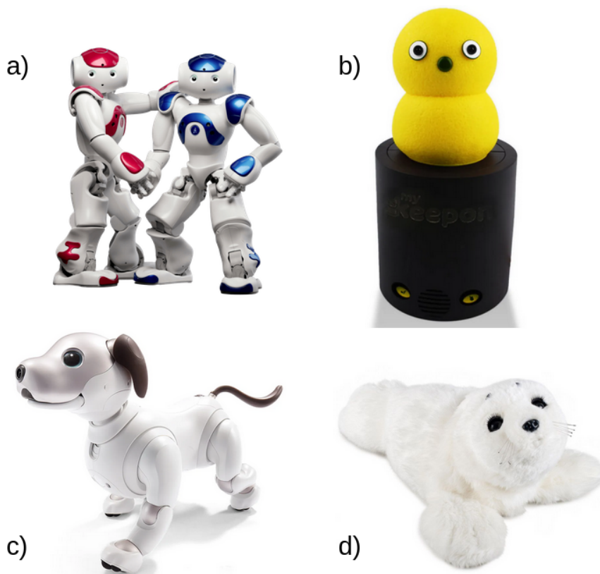
Figure 2.2: Puppet like social robots: a) Nao, b) Keepon, c) Aibo, d) Paro.
