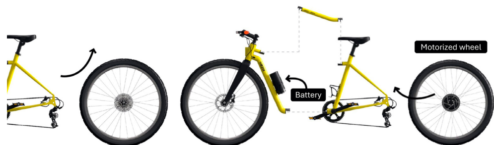
Figure 7. Transition from bike to e-bike by removing rear wheel and adding a modular bottle-battery and a motorized rear wheel.
