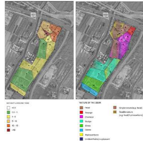
Figure 1. Examples of mapping of the product IxHT (left) and nature of the odor (right).
