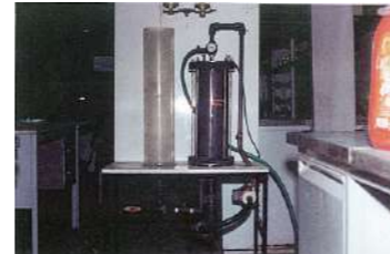
Figure 1 Pilot plant of dissolved air flotation
