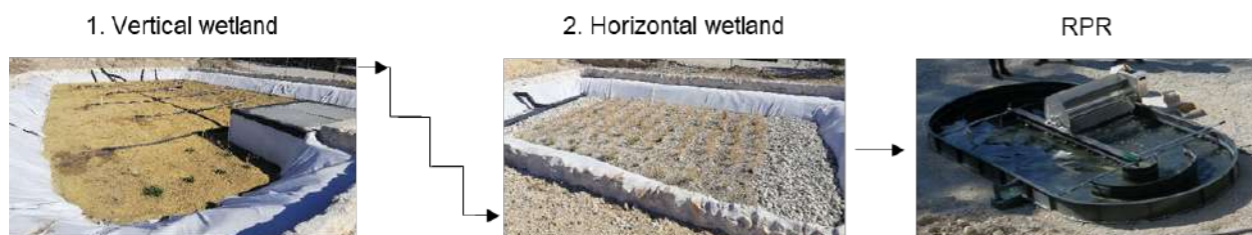
Figure 1. Demonstration system of natural based solutions coupled with advanced solar tertiary treatment in Murcia, Spain.
