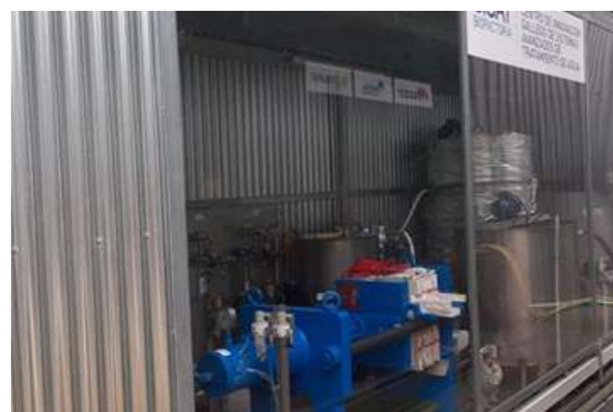
Figure 1. Pilot plant for the production of VFA operated in the project.
