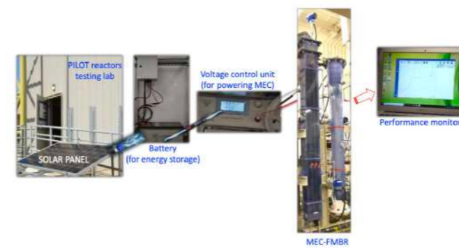
Figure 1.1 Photographs showing the pilot-scale MEC-FMBR system ( https://drive.google.com/file/d/1sLQwtwBa_AmqGQqZJaTPPhk2qWnYpV9G/view?usp=share_link ).
