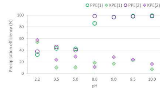
Figure 3. Phosphorus and potassium precipitation efficiency (PPE and KPE) from leachate solution. Green dots and diamonds refer to molar ratio of K:Mg:P=1:1:1, while violet ones to molar ratio of K:Mg:P=1:2:2 (2).
