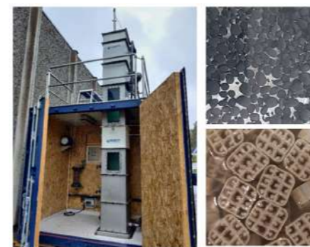
Figure 2. (a) Compact anaerobic-aerobic treatment (A2C) reactor, (b) anaerobic granular sludge, (c) aerobic biomass held in the biocarriers surface.
