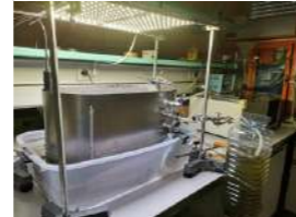
Figure 1. Stainless steel photobioreactor for microalgae cultivation with light and temperature simulation.
