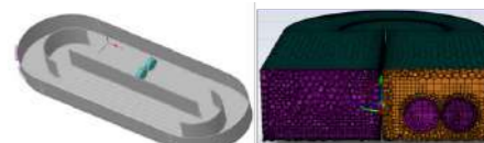
Figure 4. CFD related representations, a) Geometry of the carousel reactor of La Almunia WWTP; b) Detail of surface mesh.
