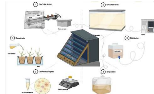
Figure 1: Experimental setup for the production and analysis of urine fertilizer from a urine evaporation module
