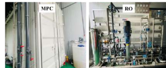
Figure 1. The configuration and photos of the pilot-scale MPC-RO system.
