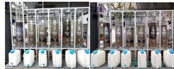
Figure 1. Small-scale VFCW after start-up with greywater (left) and after approx. one and a half years of operation (right) in Kaiserslautern, Germany.
