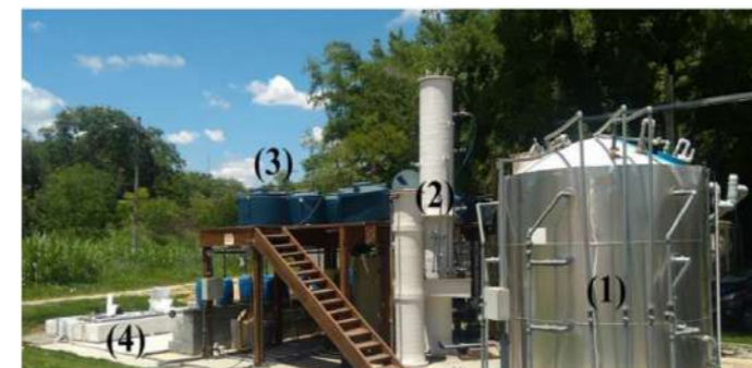
Figure 1. Waste food treatment system at the university campus (UFMG, Brazil): 1) anaerobic reactor; 2) UASB reactor; 3) solid-liquid separator and; 4) high rate algal pond.
