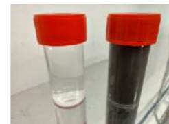
Figure 4. Comparison of the distillate and evaporation residue.
