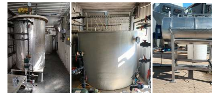
Figure 2: Pilot stages: a) Two phase anaerobic digestion, b) UF and membrane contactors, c) Solid state fermenter.
