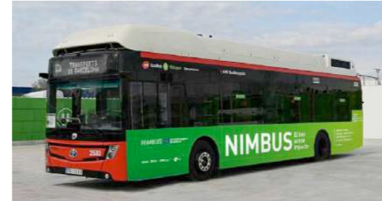
Figure 2. Public transportation bus from TMB fuelled by biomethane produced in the LIFE NIMBUS project
