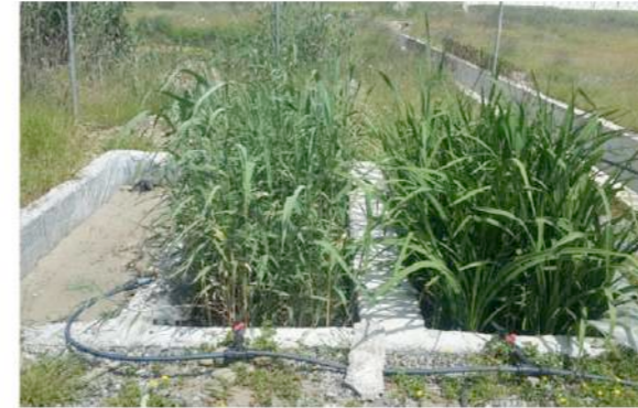
Figure3. Set up of constructed wetland built in an open field environment.
