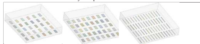
Figure 1. Three configurations of aerators in the same tank: 1) 30 rectangular plates 2) 40 rectangular plates 3) 56 rectangular narrow plates
