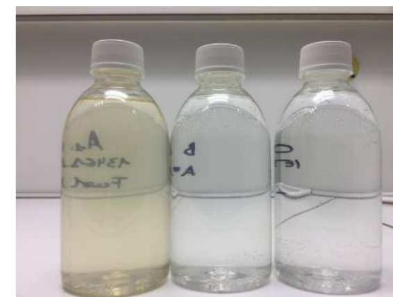
Figure 2. The resulting waters after the different treatment steps in the water reuse process: (L) UF filtrate, (M) after organics removal with activated carbon, and (R) softened process water after ion exchange, ready to be used in the full-scale industrial process.
