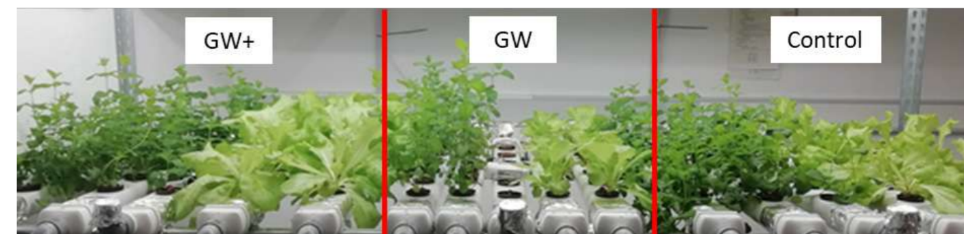
Figure 1. Hydroponic system with mint and lettuce grown in greywater plus nutrients (GW+), greywater (GW) and hydroponic nutrient solution (Control), after week 4 of the experiment.
