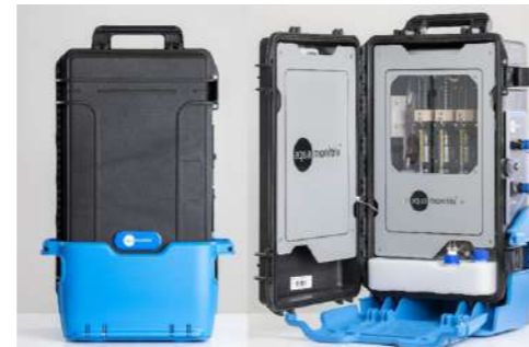
Figure 1. Aquamonitrix real-time in-situ \text{NO}_2^- and \text{NO}_3^- analyser. The exterior dimensions of the unit are 60 \times 37 \times 27 cm and the unit weighs \sim 11 kg.
