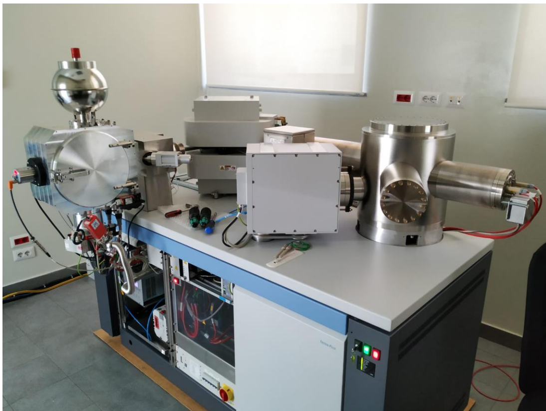
Fig. 2.4 Thermal ionization Thermo-Finnigan Triton-Plus mass spectrometer at the Radiogenic Isotope Laboratory of the Earth Science department of the University of Firenze (Italy).
