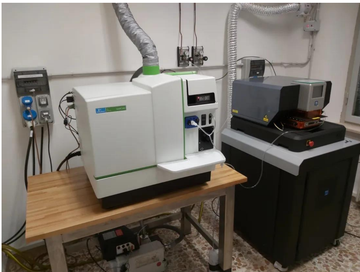
Fig. 2.8 PerkinElmer NexION 2000 ICP-MS coupled with a NWR-193 AR-F 193 nm excimer laser at the Center for Instrument Sharing of the University of Pisa (CISUP) in the Earth Science Department of Pisa (Italy).
