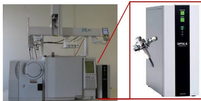
Figure 127 – GC-MS equipped with Multimode injection system inlet OPTIC4
