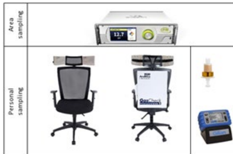
Figure 26 – Sampling strategy proposed by Dugheri et al. [70] with personal sampling conducted by two NEMO XT on the headrest, DNPH-coated cartridge with a pump and area sampling performed by a Gasera
