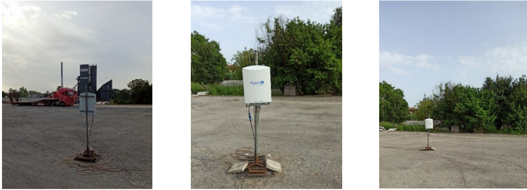
Figure 123 – PyxisGC installed between the bituminous conglomerate plant and the receptors
