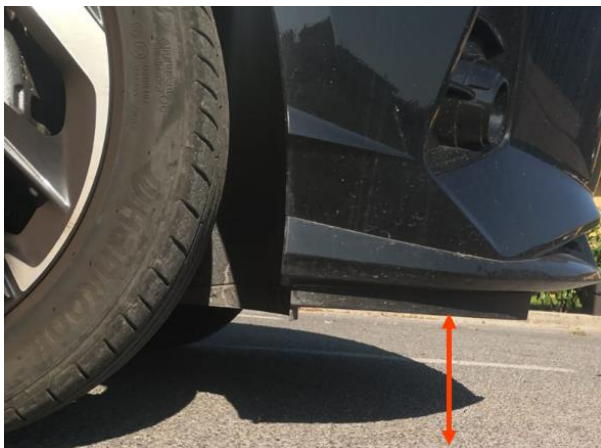
Figure 16. Air gap evaluation on the test vehicle. During the test it is assumed to be constant due to the test circuit morphology.
