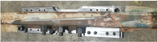
Figure 22. First prototypes of ABJ. Top: switch rails finished by milling. Bottom: assembly tests with dummy fastenings and insulating sheets.
