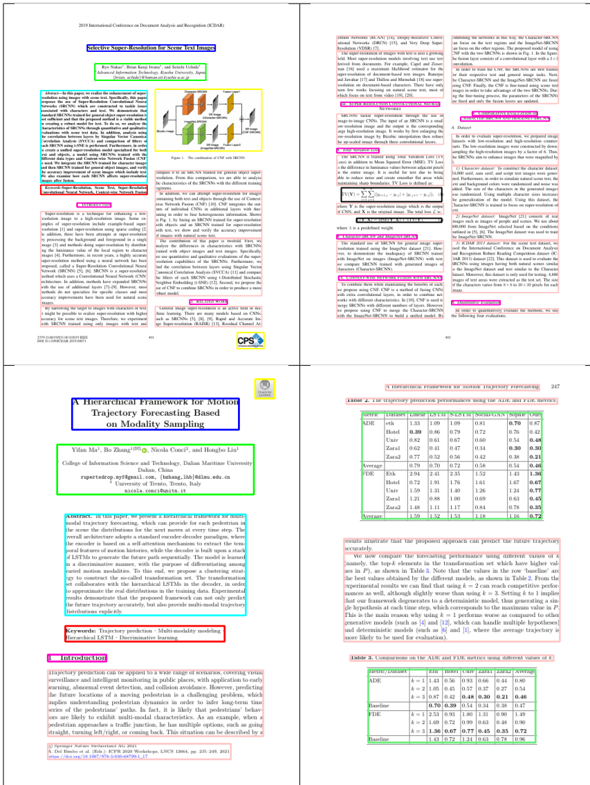
Figure 6.3: Examples of automatically annotated pages. From GROBID and PDFMiner we extract nine categories: title (blue), authors (light green), abstract (cyan), keywords (red), subtitles (purple), text (pink), images (yellow), formulas black and tables (green). Captions and references are added by hand.
