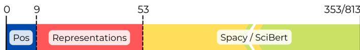
Figure 3.3: Node features: positions and representations have a fixed length; Spacy or SciBERT embeddings have a length of 300 and 760, respectively.
