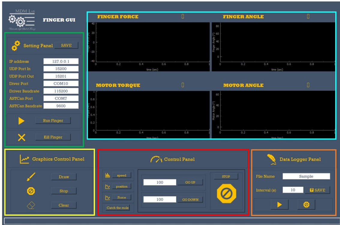
Figure 4: - An overview of the ExoGUI with colored frames highlighting the various panels. The setting panel, in green; the control panel, in red; the data logger panel, in orange; the graphics area, in blue; the graph control panel, in yellow; and the text box, in white.
