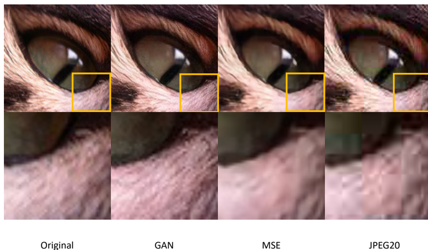
Figure 7.1: Qualitative comparison of reconstruction methods: GAN produces images more pleasant for the human eye. Best viewed in color and zoomed on computer screen. GAN: GAN-based restoration using perceptual loss. MSE: CNN-based restoration using MSE loss; JPEG 20: JPEG compression with quality factor 20.
