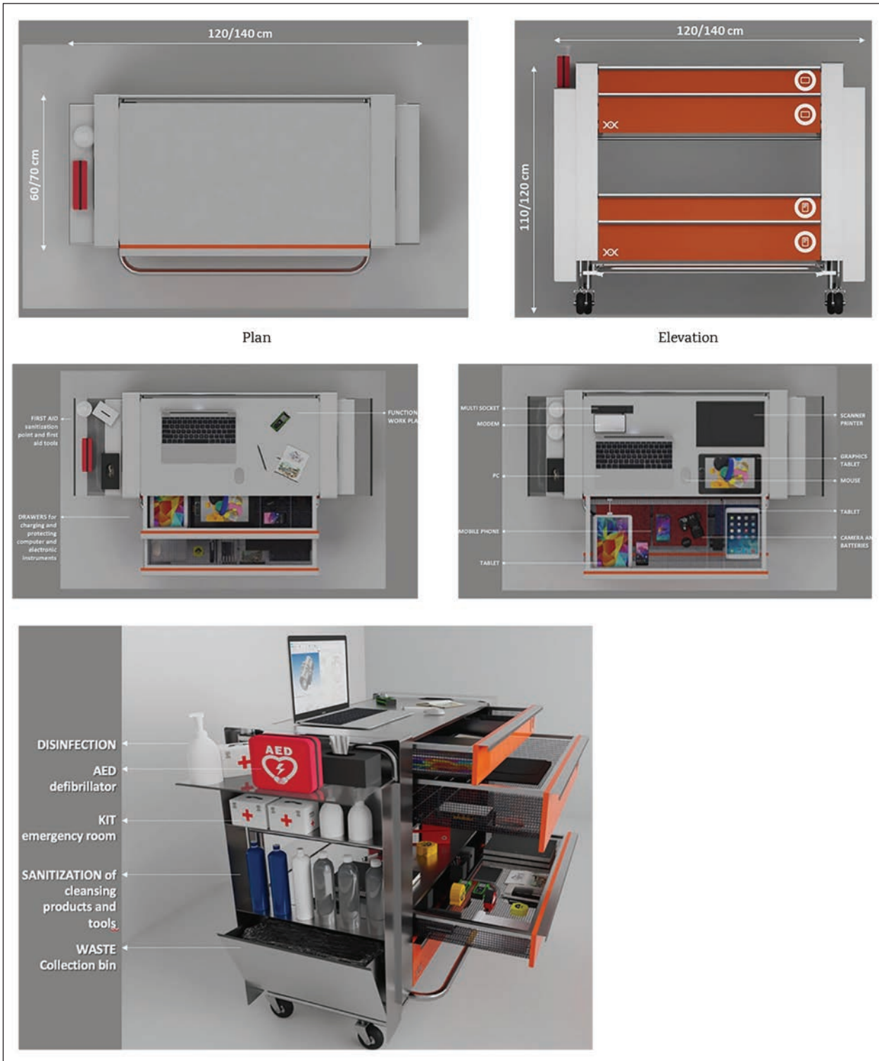
Figure 6. The DOC Construction Site Operational Desk Design
