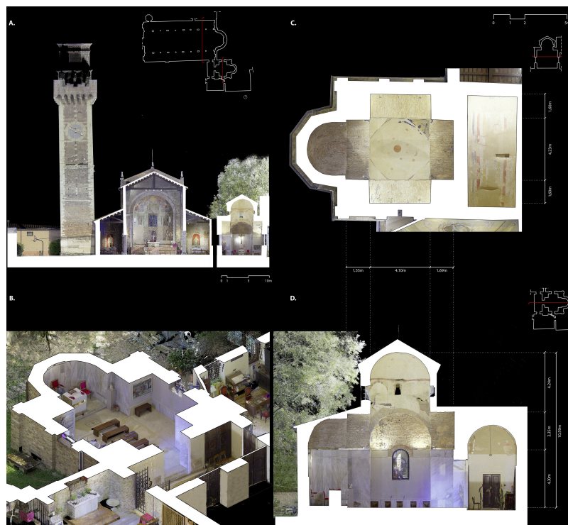
Figure 5. Analytical survey outputs of the sacellum of Santa Maria Mater Domini in Vicenza, derived from point-cloud data: (A) transverse section showing the spatial relationship between the Basilica of San Felice e Fortunato and the sacellum of Santa Maria Mater Domini; (B) axonometric section showing the plan; (C) roof plan; and (D) longitudinal section. The figure includes metric references and highlights the central domed compartment, the barrel-vaulted arms, and the relationship between the sacellum and the adjoining basilical complex. Red lines in the small reference diagrams indicate the position of the corresponding section or view.
