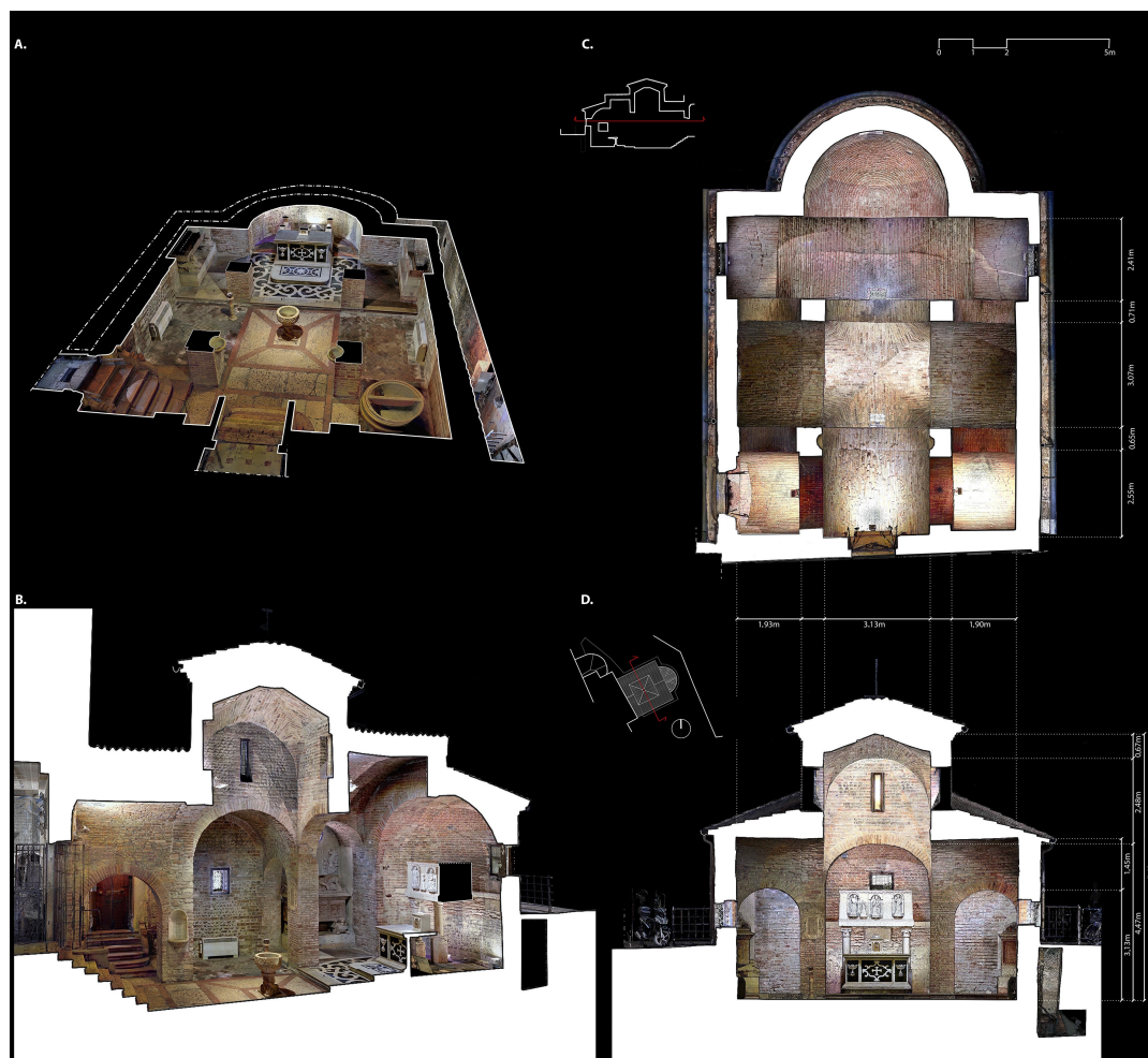
Figure 4. Analytical survey outputs of the sacellum of Sante Teuteria e Tosca in Verona, derived from point-cloud data: (A) axonometric section showing the plan; (B) axonometric section; (C) roof plan; and (D) transverse section. Red lines in the small reference diagrams indicate the position of the corresponding section or view. The figure includes metric references and emphasises the relationship between the upper wall sections, the central lantern, the lateral arms, and the architectural configuration of the monument.
