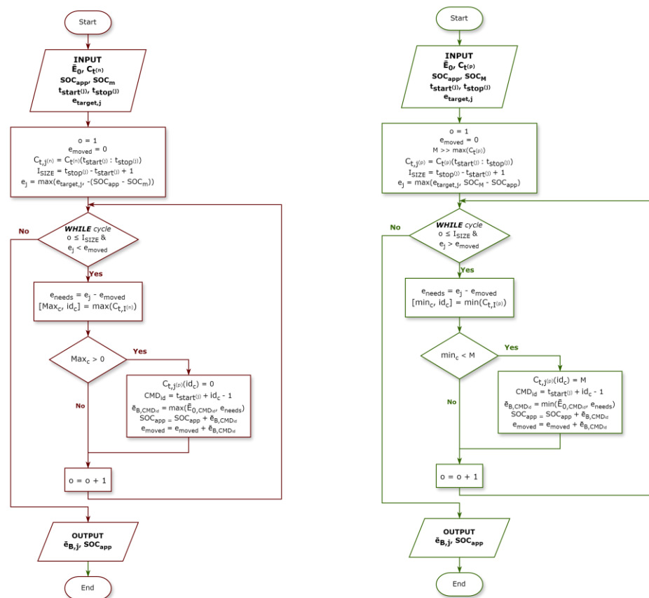
Figure 12. Operations performed in the “NEG Scheduling” block (on the left) and “POS Scheduling” block (on the right) of Figure 11.
