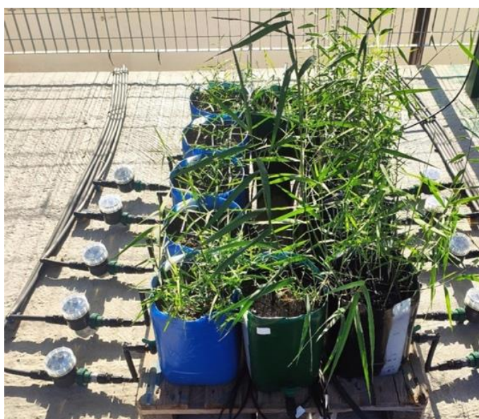
Figure SM5-1: Picture of the laboratory scale vertical flow systems at the NatLab laboratory.
