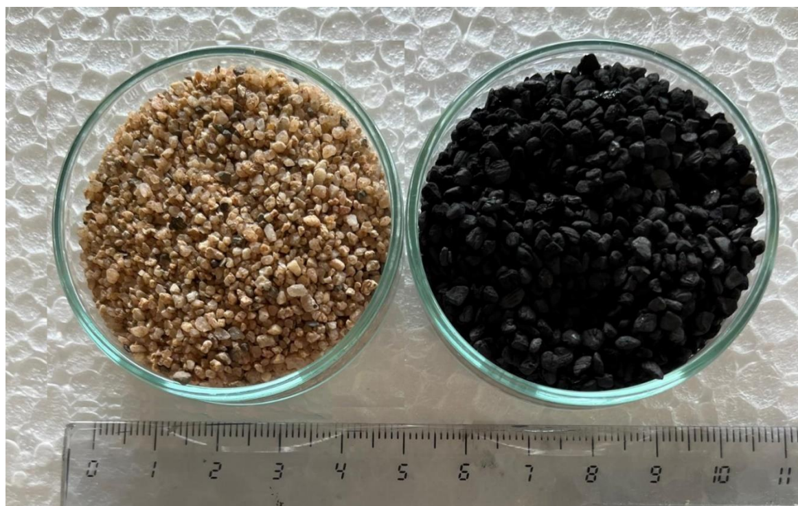
Figure SM2-5: Picture of the sand and the biochar produced from olive pomace used in this study.
